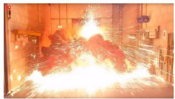
In addition, pressure waves generated by an arc flash explosion can carry a force up to thousands of pounds per square inch, which is powerful enough to knock down or throw nearby workers, and cause damage to the eyes, eardrums, lungs, brain, and other organs. These pressure waves are commonly known as an 'arc blast.' The force created from the blast can exceed a 'tonne' of pressure per square inch and can be fatal up to distances of 3 meters.
