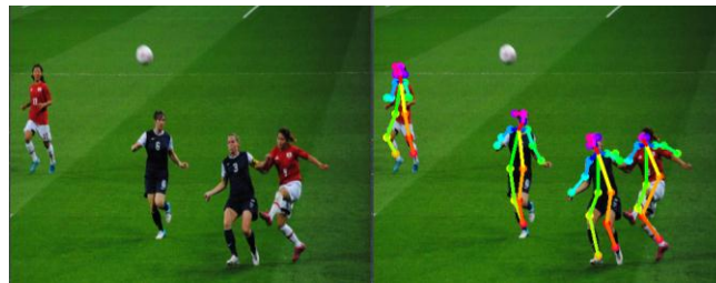
Figure 8. Input vs. Result of the Pose Estimation of a Multi-Person View Image
