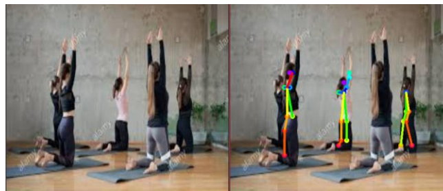
Figure 7. Input vs. Result of the Pose Estimation of a Multi-Person View Image
