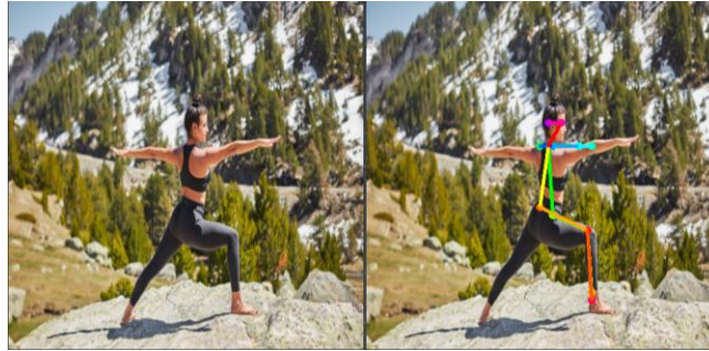
Figure 6. Input vs. Result of the Pose Estimation of Side Body View Image
